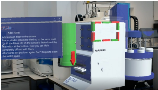
Fig. 5. HoloLens recognized the image, and the multi dosage unit was precisely overlapping with the real one. The position of the target image was framed by green and red rectangles. For guiding the user to the filters, a green cylinder covered the filters in this step. An arrow shows the switch to put off the filter stack.
