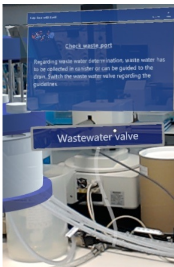
Fig. 6. The tooltip anchored to the wastewater valve, that needs to be switched in this step. The panel contains additional information on when and how the valve should be switched.
