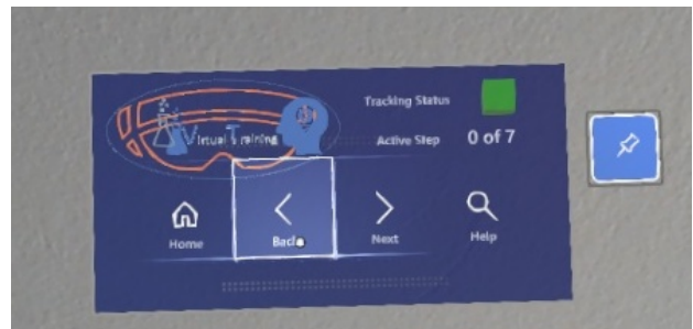
Fig. 7. Near interface panel with the registered image. Users can change the steps with the two buttons in the middle. The help button opens the panel with information, a home button switches to the start scene.
