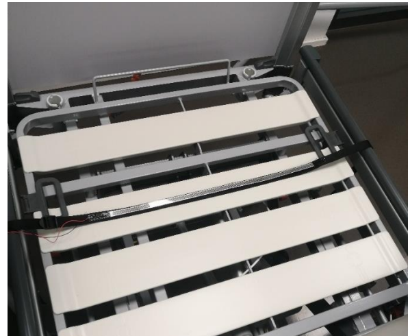
Fig. 4. The Force membrane sensor was sewed on a nylon belt which can be fixed on the bed stead. This allows the sensor to be placed in multiple ways and on various beds.
