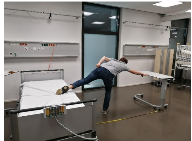
Fig. 7. The setup to evaluate the effectiveness of the sensor and the detection by a threshold consist of a hospital bed with build in sensor and a table on which sweets will be placed. The participants are challenged to get some of the sweets without the sensor detect that they are leaving the bed. For this the table is placed out of reach from the bed.
